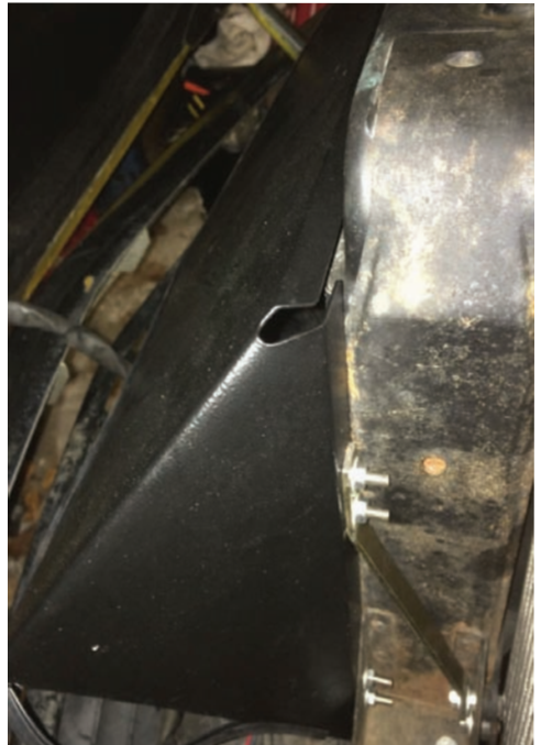
Picture 9. Radiator Shroud/Cowl in Powder Coated Aluminium
