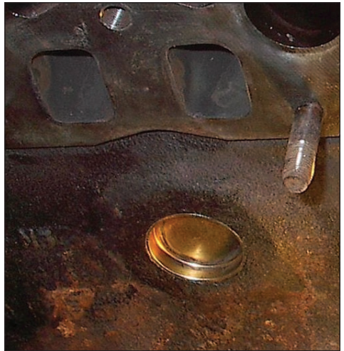
Picture 7 New Core plug fitted.
