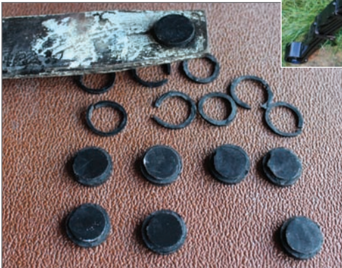
Photo 4: Spring thrust pads and where they fit
