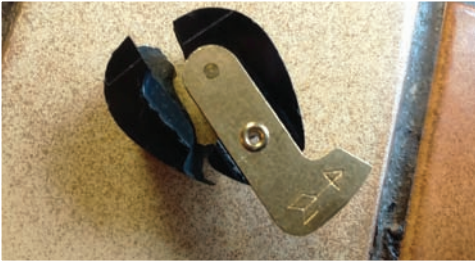
The offending rotor arm, now very definitely broken!
