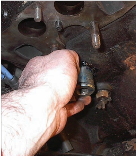
Picture 6 Getting ready to drift new core plug into place using a socket.
